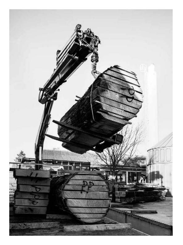
Whenever shelter trees are felled we take them immediately to the saw mill to be cut into 3, 4 and 5 inch planks. The freshly cut planks are then brought directly to our workshop. While the planks are still naturally moist we cut out and pair the raw pieces needed for a particular chair.
