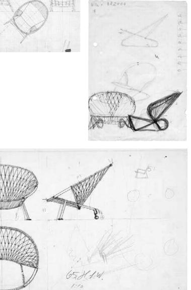
Wegner's first sketches bear a clear relationship to the **Peacock Chair** but later variations became more geometrical and made use of steel and flag line. The distinctive pattern created by clamping the flag line with metal clips appears on sketches drawn in early 1960 and the first drawings of the **Circle Chair** are dated 1965.
