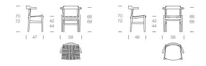
**pp68** | **pp58** is optimised to be practical. The short armrests makes it easy to enter and move around the chair. It fits well underneath the table and can also hang from the table top to make cleaning easier. The all solid wood tenon joints have been tested to withstand one ton of pulling strength. The combined arm and backrest is made of one piece of solid steam bent wood. **pp58** comes with an upholstered seat in either fabric or leather.
