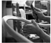
The **Chinese Chair** is one of Wegner's earliest designs in production yet it is produced using the most modern bending technique. A single piece of steamed solid wood is compressed along its length using an advanced technical process and is immediately rounded before it is bent in three dimensions. Bending a round piece of wood would appear to be simple, but because of the complexity of the bend, it requires advanced tools, specialised knowledge and experience to control the operation.
