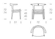
The armrests are always cut from the same piece of wood, so the grain will match. The joint detail in the back is made of rosewood.
