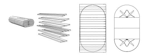
The composition of each tabletop is always thoughtfully considered and planned in detail. Every section is carefully evaluated from what a tree offers and they are glued together in the exact order selected by the individual craftsman for a particular top.
