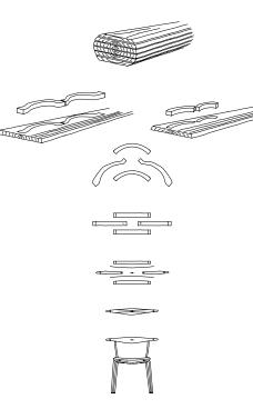
The **Minimal Chair** seeks to provide an adequate support for the back with the minimum use of wood. Four pieces of solid wood are carved from 1¾ inch planks cut from trees around 100 years old. The right and left armrests and the lower and upper centre sections are always cut in line of one another and paired. The arched construction requires three different directions of wood grain with long gluing surfaces to ensure sufficient strength.
