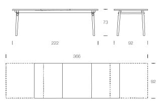
**pp850** comes with four solid wood leaves included. The main tabletops are primarily made of plain cut wood, and the leaves are primarily made of quarter cut wood. The leaves come in two different widths for convenience and flexibility.
