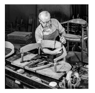
In the 1950's and 60's when the **Round Chair** were made at Johannes Hansen's workshop the shaping had to be done by hand starting with just a raw cut piece of wood. This resulted in many different 'versions', some of which varied significantly from the original design both in terms of shape, strength and comfort. At PP Møbler we take very seriously the subtle details in the organic shapes of Wegner's finest designs.
