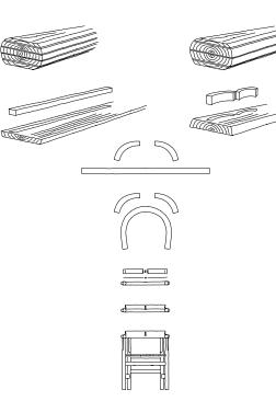
The **Ferry Chair** combines a length of steam bent wood with two pieces of solid wood cut from a 2½ inch plank in line of one another and paired. This sophisticated construction provides a comfort similar to that of the **Round Chair** but can be made using trees that are about 100 years old.
